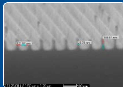
Imprinted grating pattern with 25nm line width and 120nm period.
